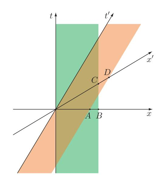
An inertial observer O' carries a ruler of length  $L_0$  at speed v past an inertial observer O.
